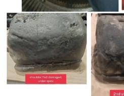
1st shoulder pad also damaged under spec both never replaced
